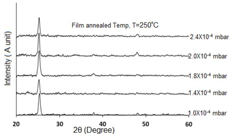
**Fig. 3: Partial O<sub>2</sub> effect on V-TiO<sub>2</sub> films of XRD spectrum at 250° C.**
