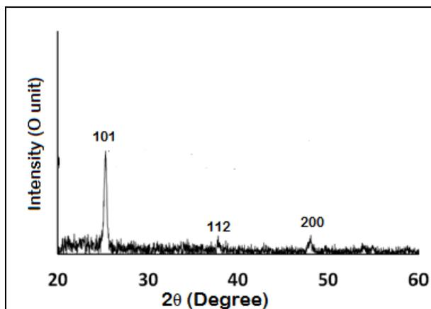
**Fig. 1: XRD pattern of TiO<sub>2</sub> at 100° C.**
