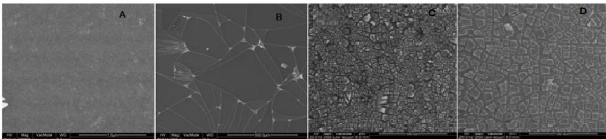
**Fig. 5: SEM micrographs of V-TiO<sub>2</sub> films at (A): 100°C; (B): 150°C; (C): 250°C; (D): 350°C.**
