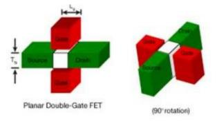
FinFET device provides better short channel control by its fully depleted behavior with the need of less or no doped channel. This les doped channel lowers the scattering of lower dopant ion resulting improved drive currents and less random dopant fluctuations (RFD). This research aims on issues raised on technology & circuit design.[6]
