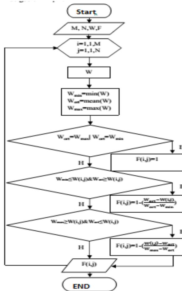
Figure 1: Adaptive fuzzy filter flow diagram.
