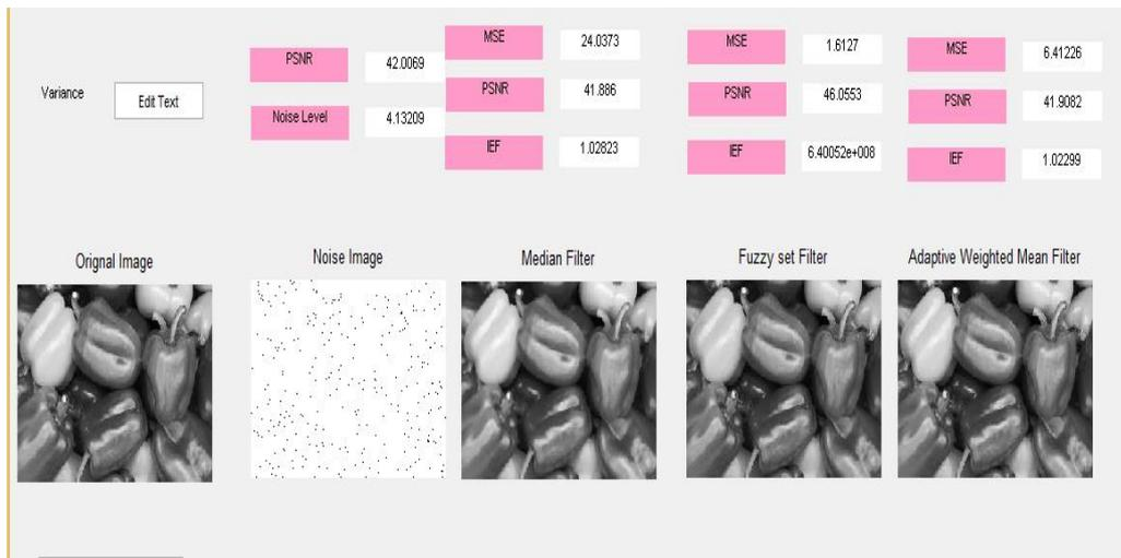
Figure 3 Comparison of Noise level & Median Filter ,Adaptive weighted filter and Adaptive Fuzzy Filter
