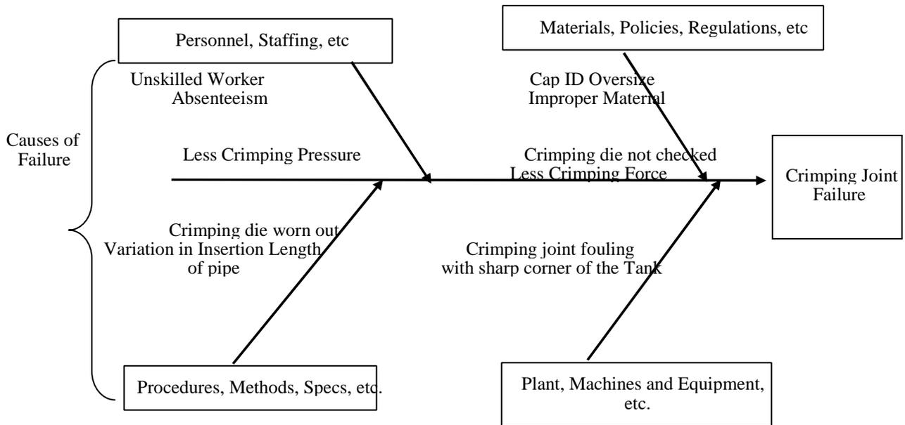
The Taguchi methodology is used to discover an ideal solution to the causes of dismissal. Three primary faults: Less Crimping Depth, Hose Length Variation and Cap Inner Diameter (Oversize) are regarded for the Crimping Leaking of the Hose Pipe Assembly.
