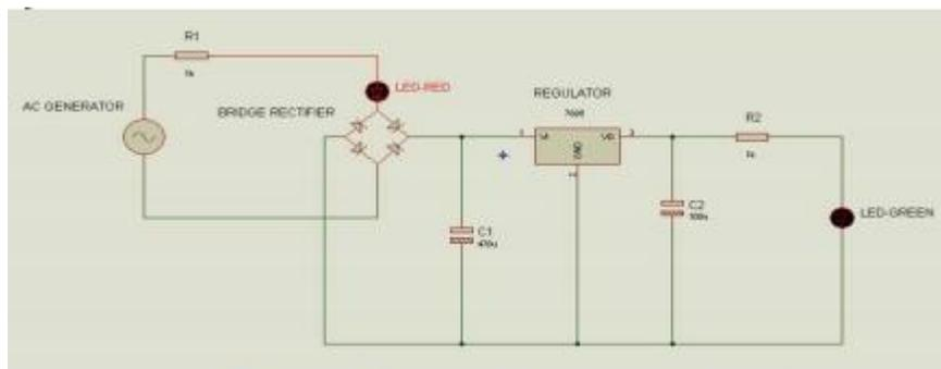
Figure 11: AC to DC conversion circuit
