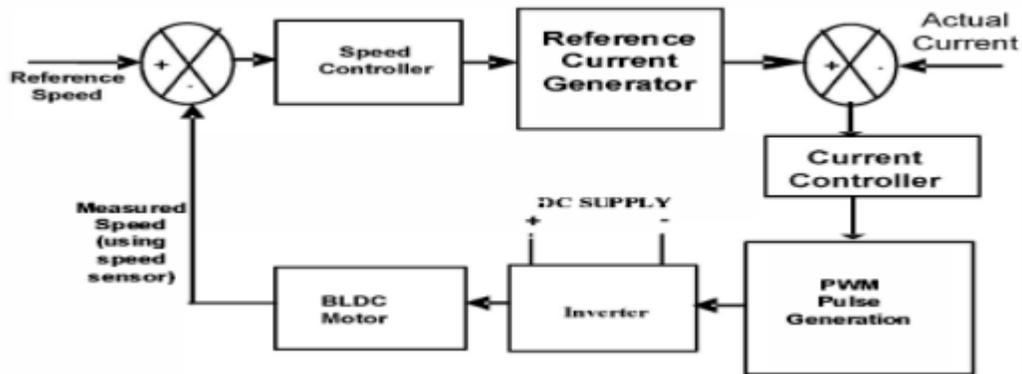
**3. ANFIS Speed Controller-** ANFIS Controller does not require a mathematical model of the system and it works on a structure prepared from the knowledge base. In ANFIS Speed controller the inputs used are the speed error and rate of change of speed error.
