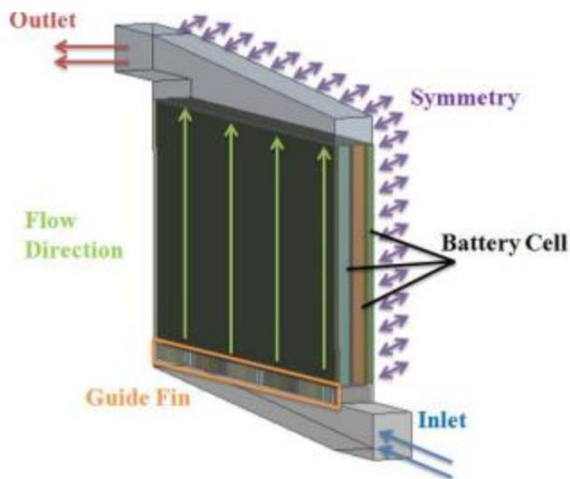
**Figure 2(a).** Configuration of Battery Module Analysis Model.
