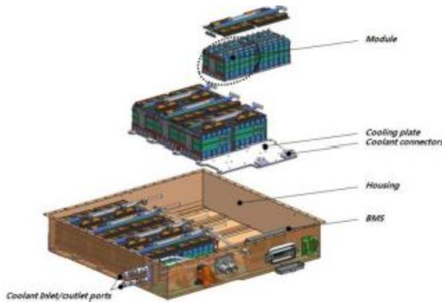
**Figure 1.** Configuration of Battery Pack System.
