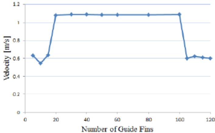
**Figure.** Comparison of Average Velocity by Number of Guide Fins in All Cooling Channels
