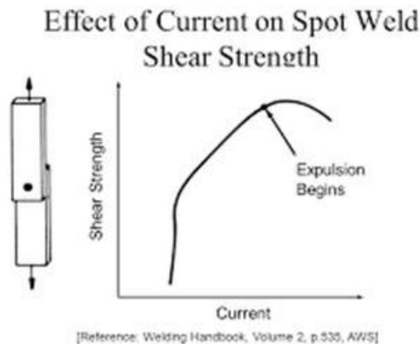
Fig-3: Graph between shear strength and Current
