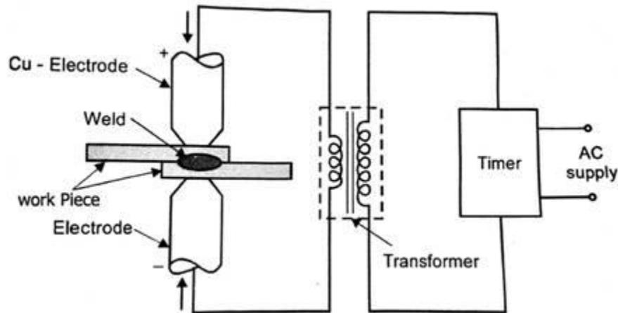
Fig-1 Schematic View of Resistance welding
