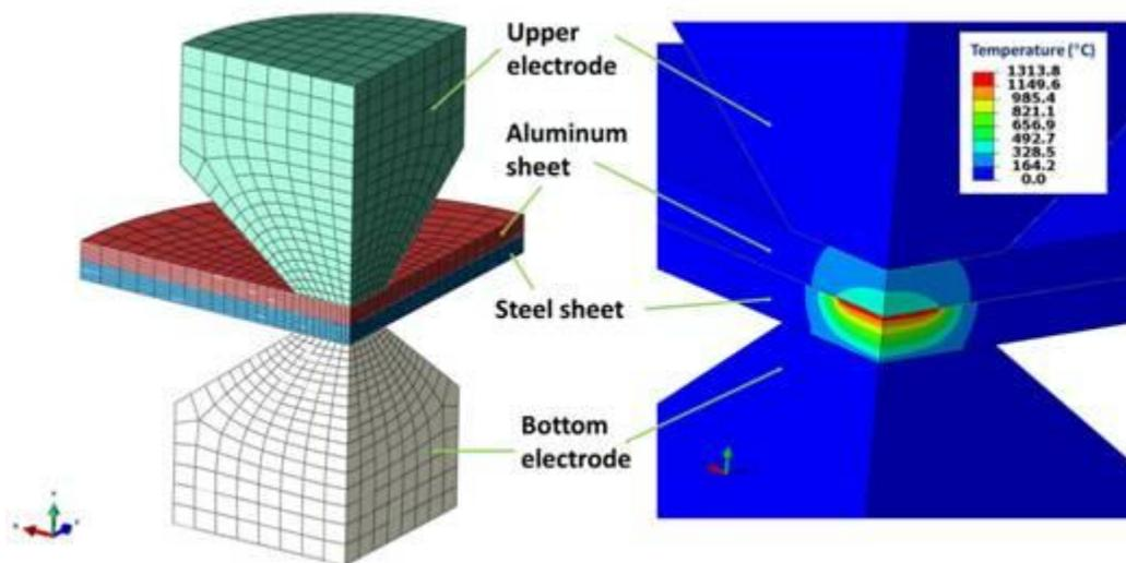
Fig-2 FEM View of Resistance welding
