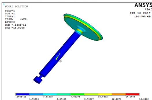
FIG. 4: THERMAL FLUX OF VALVE SEAT – EN21-4 STEEL
