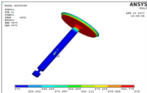
FIG. 2: TEMPERATURE OF VALVE SEAT EN21-4 STEEL
