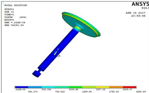
FIG. 3: THERMAL GRADIENT OF VALVE SEAT – EN21-4 STEEL
