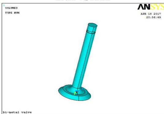
FIG. 5: BI-METAL VALVE OF VALVE SEAT – EN21-4 STEEL
