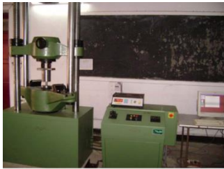
Figure: The experimental set-up mounted on UTM for extrusion
