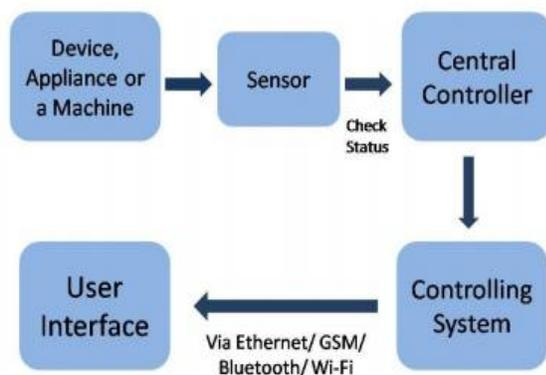
**Figure: Basic architecture of a Home Automation System**
