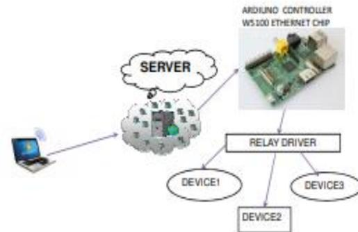
This complete system has two parts. One is web page to control and other is the appliance to be controlled like motor, bulb etc. The web page consists of the login page, which is used for authentication of a particular appliance to particular user. Once we logged into it we can control the
