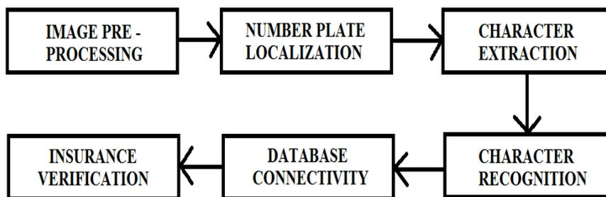
Figure.1. System flowchart of license plate recognition
