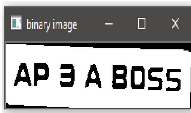
Figure.4. Output of Otsu's Method
