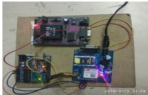
Figure.8. Attendance system based on GSM technology on 8051 Micro controller.
