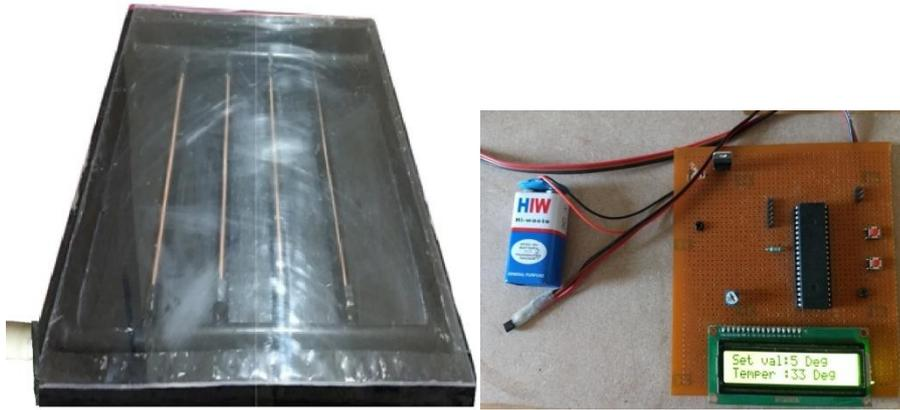
**Fig. 2 The experimental arrangement of the solar cavity collector**
