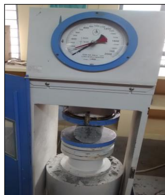
Fig. 4 Split Tensile Strength Test on Cylinder
