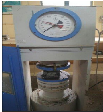
Fig. 3 Compressive Strength Test on Cube
