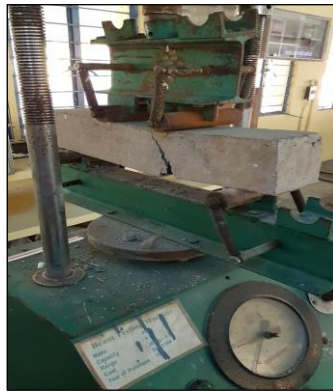
Fig. 5 Flexural Strength Test on Prism
