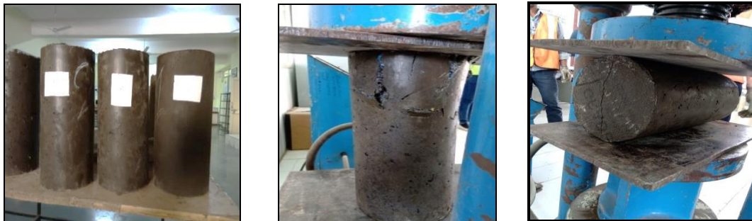
Figure no.1. a) Demoulded Test Samples B) Failure under Compression Testing C) Failure under Split Tensile Testing
