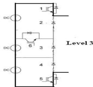
**Figure 6. Level 3 =  $3 V_{dc}$**
