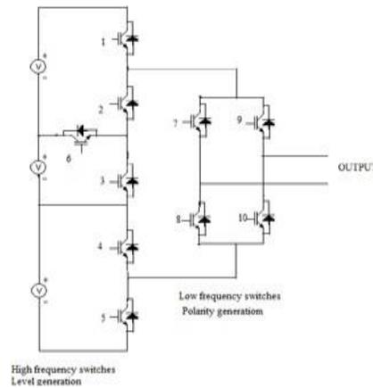
**Figure 1 General single phase multilevel inverter (using reverse voltage topology) circuit**
