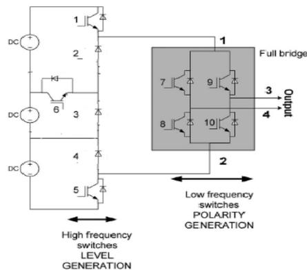
**Figure 2 Proposed circuit using RV topology**
