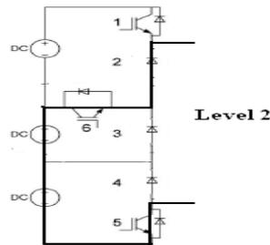
**Figure 5. Level 2 =  $2V_{dc}$**
