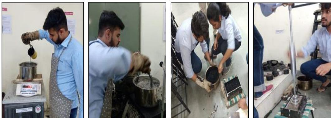
**Figure 2. a) Pouring of bitumen b) Mixing of materials, c) Filling of mould
