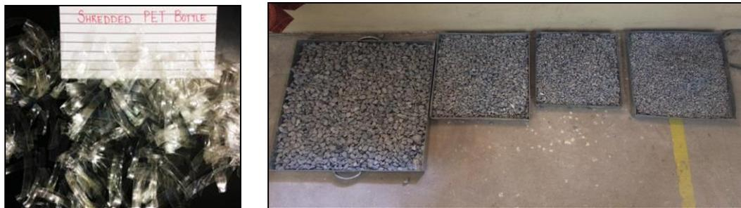
**Figure 1. a) Shredded PET Bottles b) Recycled Concrete Aggregates- 12.5mm, 10mm, 8mm, and 6mm (from left)**
