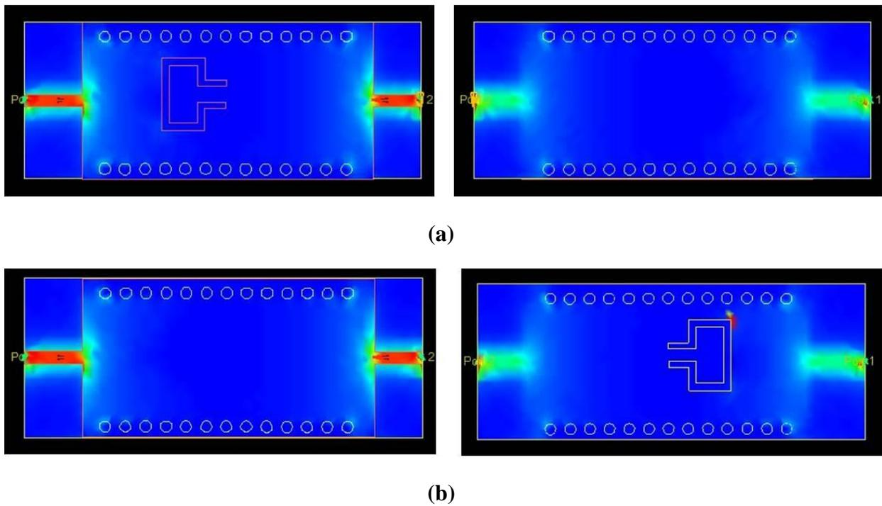
**Figure.7** Electromagnetic field distribution of the filter
