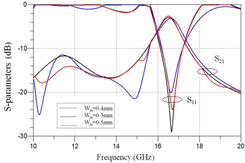
**Figure.6** Frequency response of the filter with L-slot on bottom layer with varying slot width
