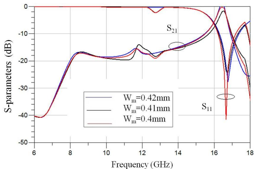
**Figure.5 Frequency response of the filter with L-slots on the top layer with varying slot width**
