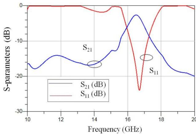
Figure.4 Simulated S-parameters of the filter with L-slots on bottom layer
