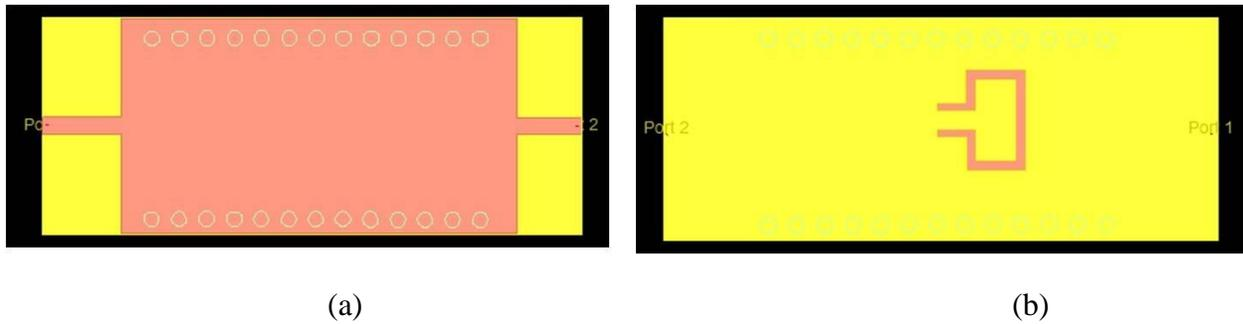
Figure.3 Layout of the SIW with L-slots etched on the bottom of the substrate
