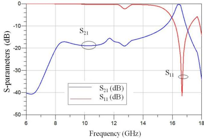
Figure.2 Simulated S- parameters of the filter with L-slots on top layer
