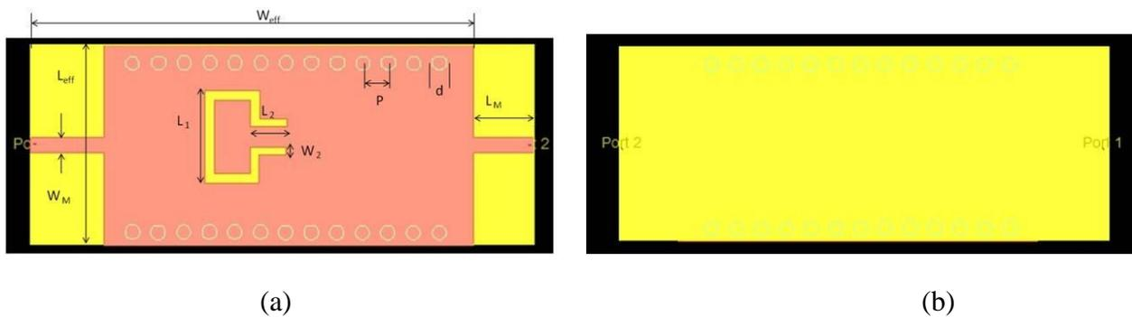
Figure.1 Layout of a SIW with L-shaped slot on the top of the substrate side
