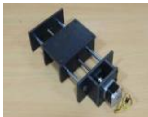
Figure 12. Z axis assembly
