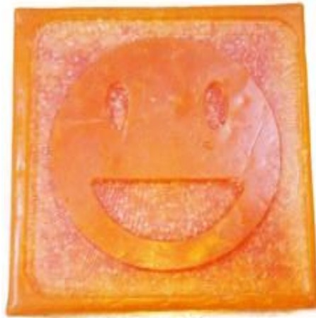
Figure 22. Sample product milled in wax using CNC mill prototype
