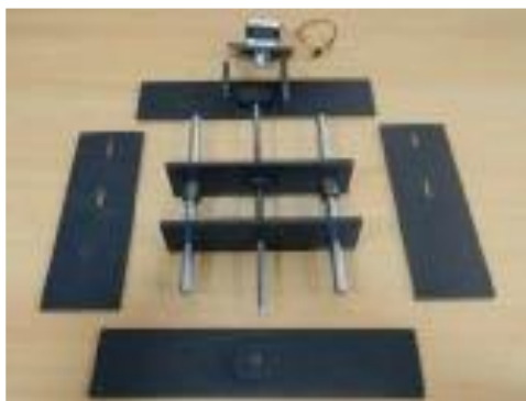
Figure 9. Y axis assembly exploded
