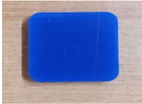
Figure 20. Sample product milled in plastic using ShopBot Desktop D2418
