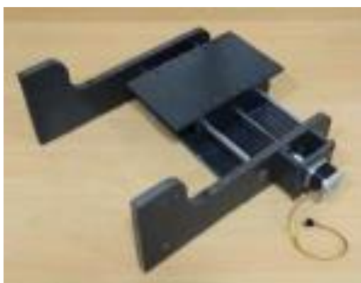
Figure 11. X axis assembly with column
