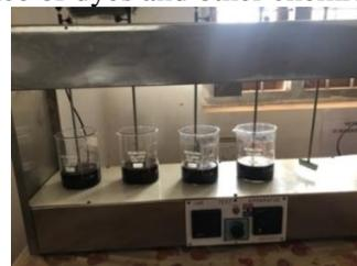
Fig 4. Batch adsorption studies on textile effluent
