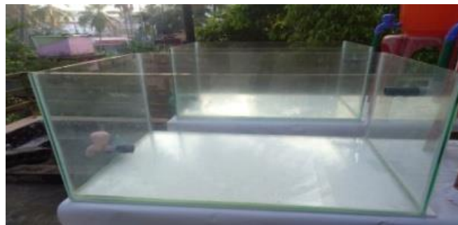
Fig no.2 Glass basin with slope provided
