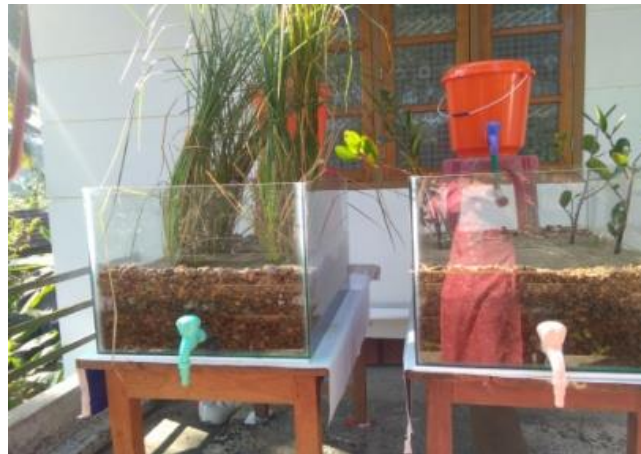
Fig no.5 the constructed wetland unit which is filled with water for plant growth
