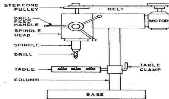
Figure.1 Drilling machine setup
