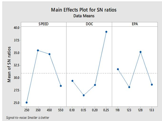
Fig: 8 SN ratio graph for diameter error
