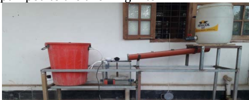
Fig.37 Experimental set up for small scale model for PWWs
