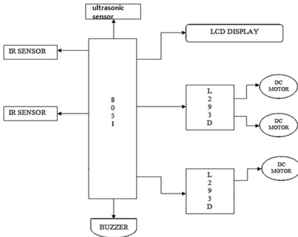
Fig.1 : Block Diagram of Microcontroller based Driverless Metro train
