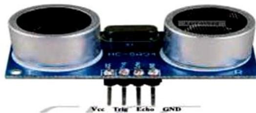
**Fig.3: Ultrasonic Sensor**
