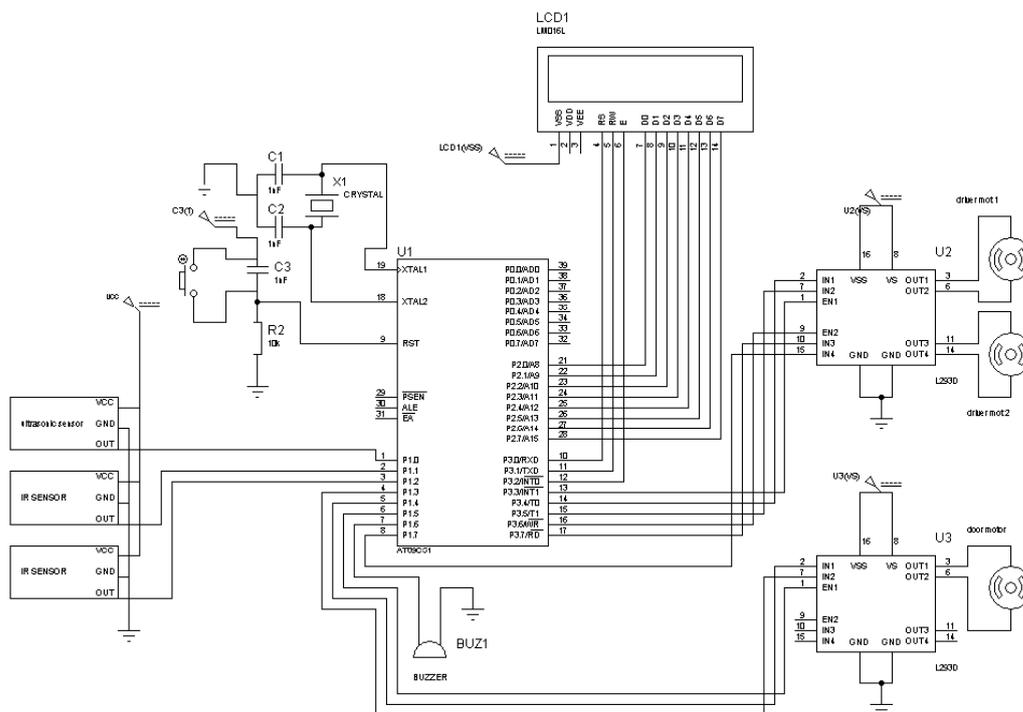
Fig. 5 Schematic Diagram of Microcontroller based Driverless Metro train
