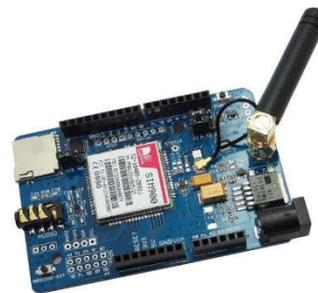
Figure 2: GSM Modem
