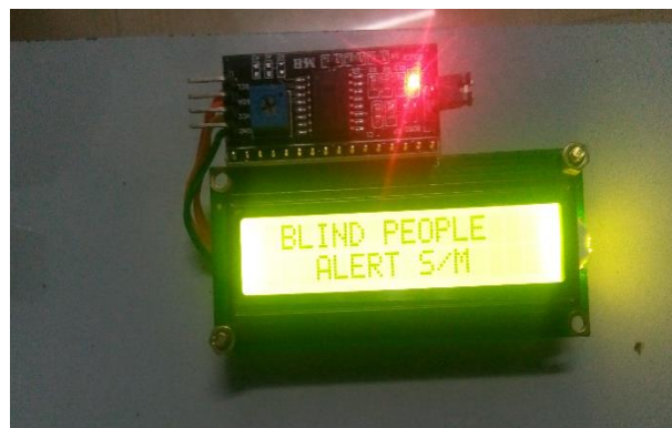
Fig. 4.2 LCD Display for Blind people alert system
