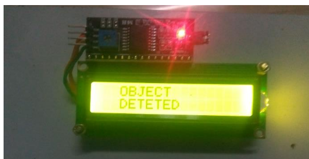
Fig. 4.2 LCD Display for Blind people alert system
