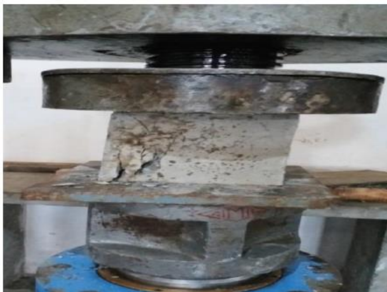
Fig. 4: Cube fixed in CTM to determine compressive strength.
