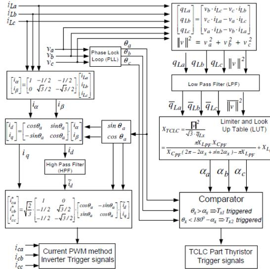
Fig. 5. The control block diagram of hybrid-STATCOM.
