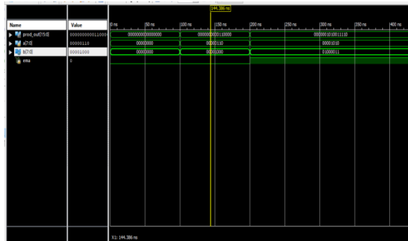
Fig.14 Simulation result of proposed Approximate DQ4:2C4 compressor implemented in 8 bit dadda multiplier
