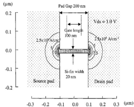
Fig. 12 Simulated current density contours in the poly-Si S/D pads. The fast spread of the current indicates effective reduction of the series resistance
