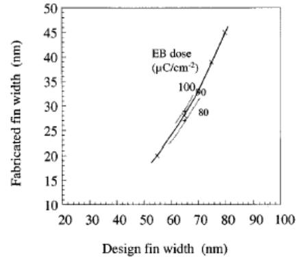
Fig. 11 Relationship between designs Si-fin width practical size with EB dose as a parameter.
