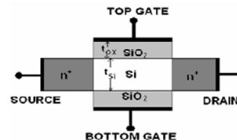
Fig. 1: Cross section of a generic planar DGFET [5]
