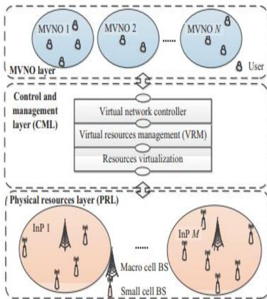
**Fig: A virtualized small cell network architecture**
