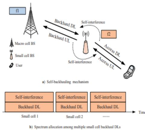
Fig:A small cell self-backhauling mechanism based on full duplex communications.
