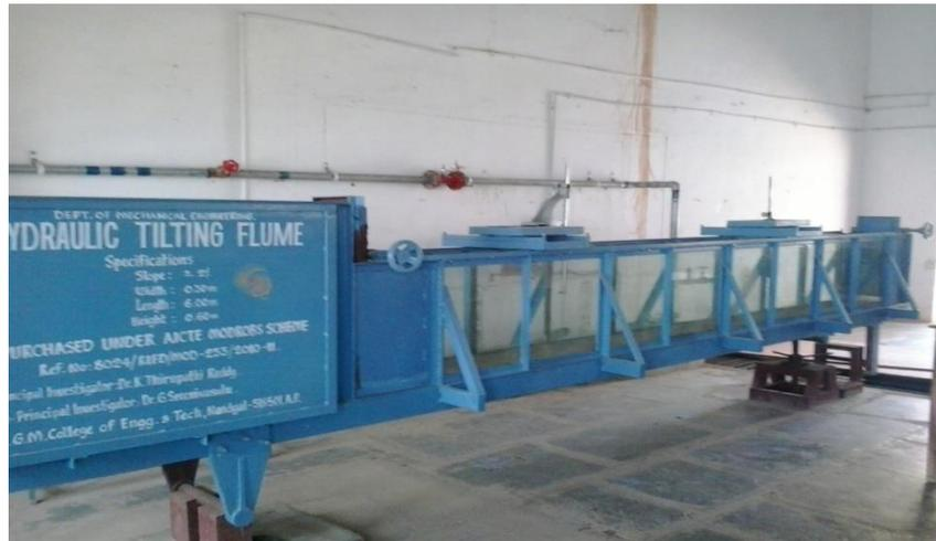
**Fig 6.1: Hydraulic Tilting Flume**
