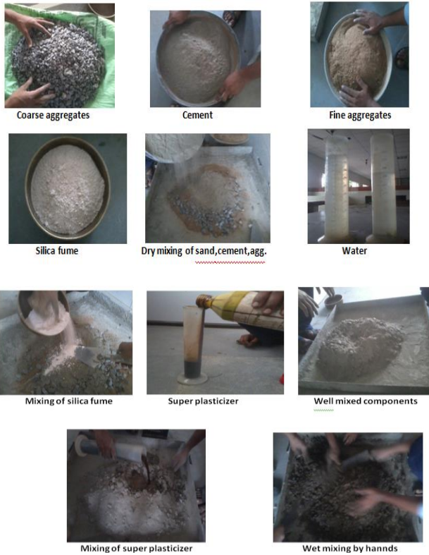
Fig. 4 making of concrete by hand mixing
