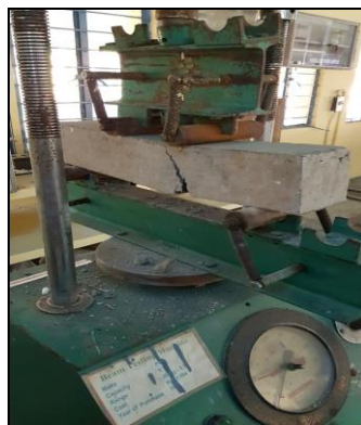
Fig. 5 Flexural Strength Test on Prism
