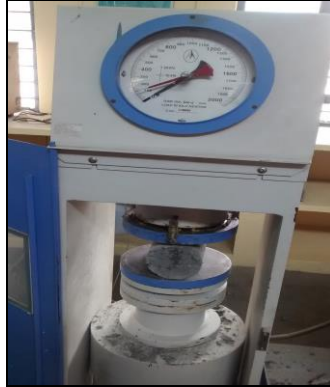
Fig. 4 Split Tensile Strength Test on Cylinder
