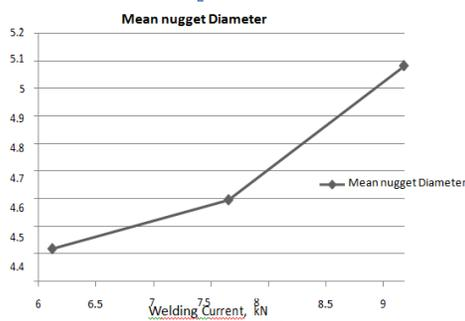
Nugget diameter increases with increase in welding current and when welding current is 9.18kN nugget diameter is 5.09 kN.
