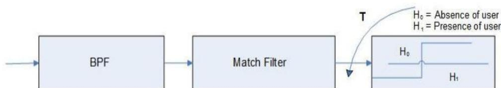
Figure 4: block diagram of matched filter detection
