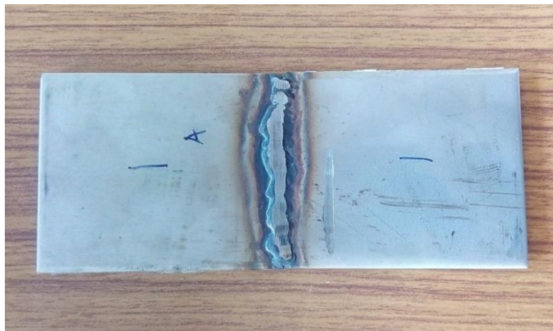
Figure.3 Stainless Steel 316L plates after welding
