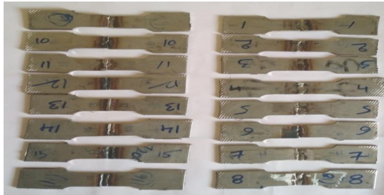
Figure.6 Welded Pieces after UTM Test
