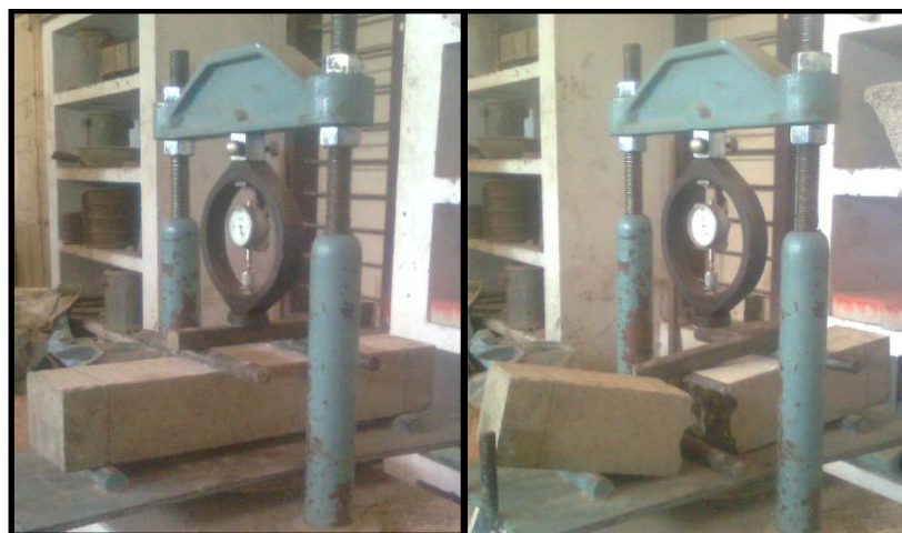
Figure 5: Flexural strength test on beams
