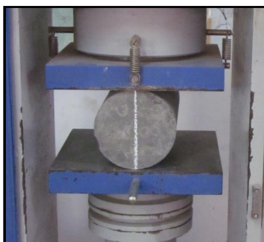
Figure 3: Split tensile strength test on cylinders
