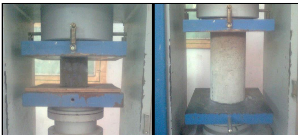
Figure 1: Compressive strength test on cubes and cylinders
