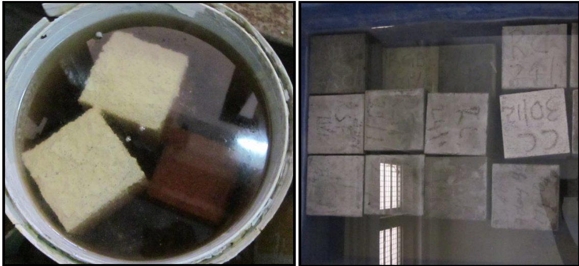
Figure 7: Specimens exposed to sulphuric acid and sulphate attack
