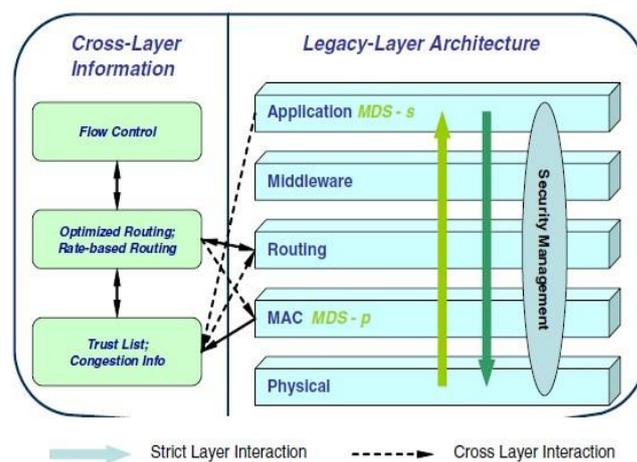
**Figure 3. Frame Work for Cross-layer system to handle MAC misbehavior [26]**
