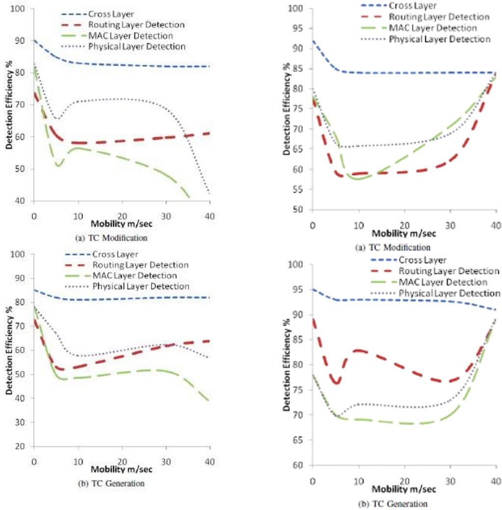
Figure 4. Simulation results for TC based detection: True Positives and Negatives
