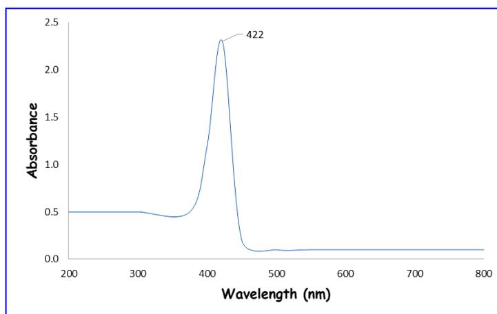
**Fig.1: UV-Vis absorption spectrum of silver nanoparticles synthesized by treating 1mM aqueous AgNO<sub>3</sub> solution with *Dodonaea angustifolia* leaf extract after 5 hrs.**
