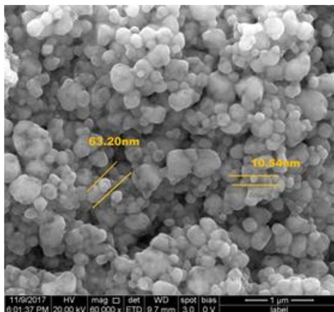
**Plate.2: High resolution scanning electron microscopic (SEM) image of silver nanoparticles (AgNPs). Polydispersed (Cluster) AgNPs ranged between 13–63nm.**
