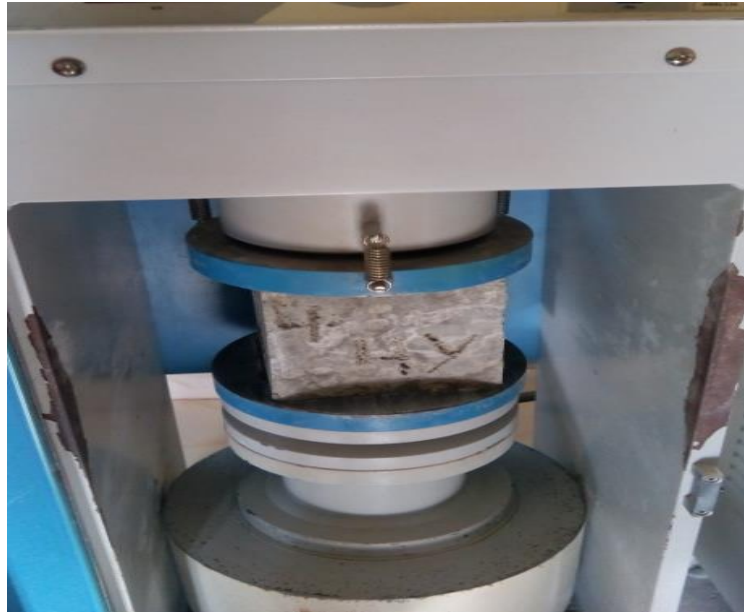
Fig 7 Testing of compressive strength of Cube
