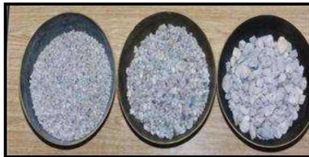
**Figure 3. Recycled Coarse Aggregate**
