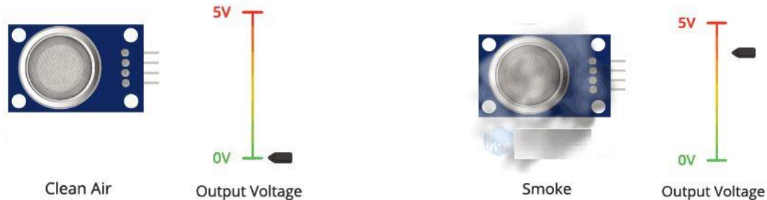
Fig3. Smoke Detection by Using MQ2 Sensor
