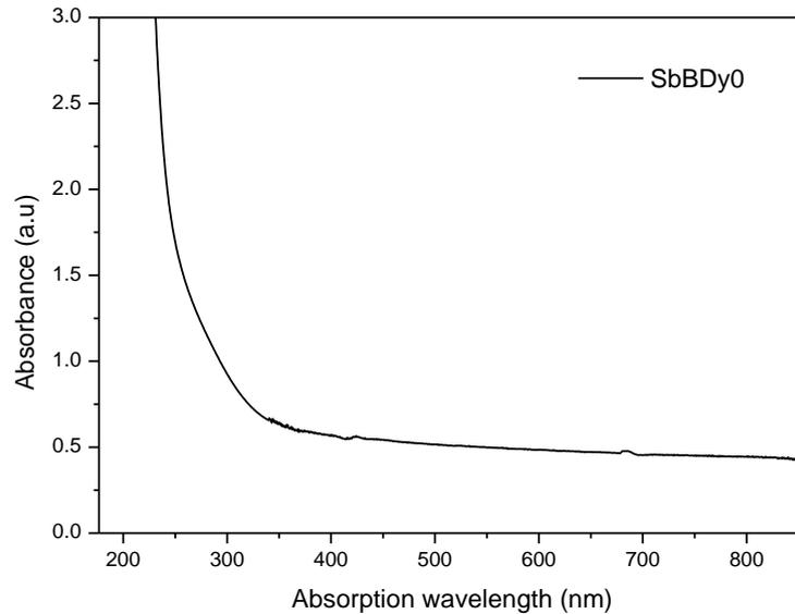
Fig. 1A Optical absorption spectrum of SbBDy0 glass
