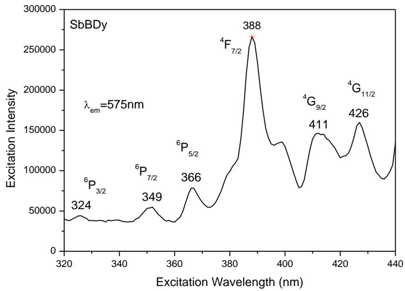
Figure 3 Excitation spectrum of SbBDy0.5 glass monitored at 575nm wavelength
