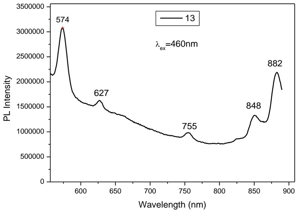
Figure 6 Emission spectrum of SbBDy0.5 glass at 460nm excitation wavelength
