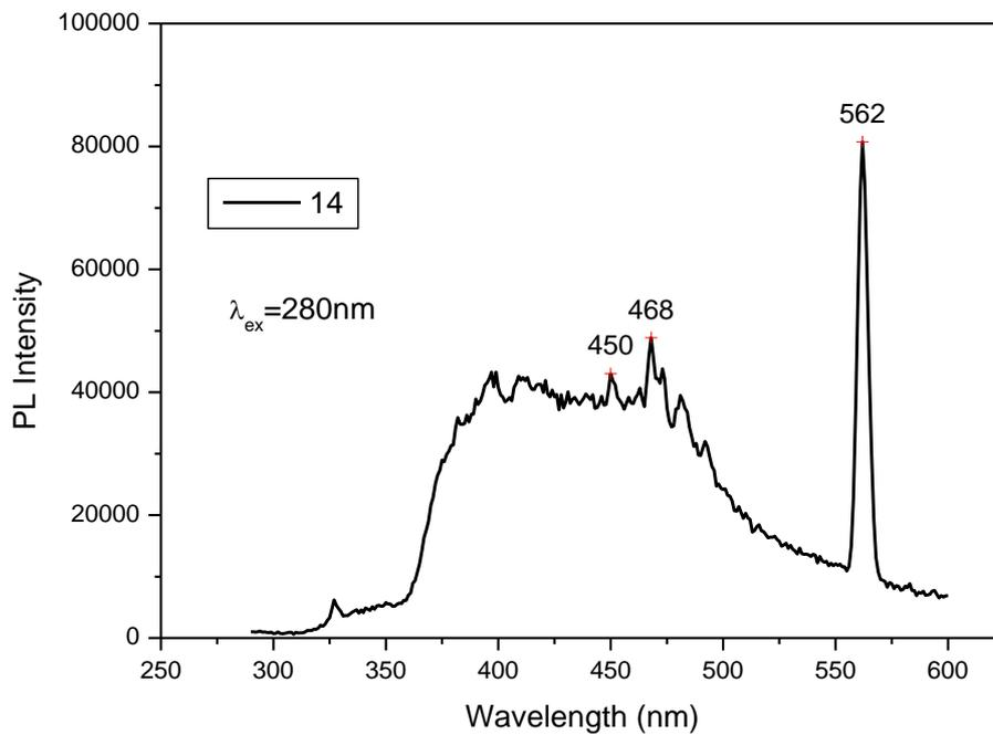
Figure 4 Emission spectrum of SbBDy0.5 glass at 280nm excitation wavelength
