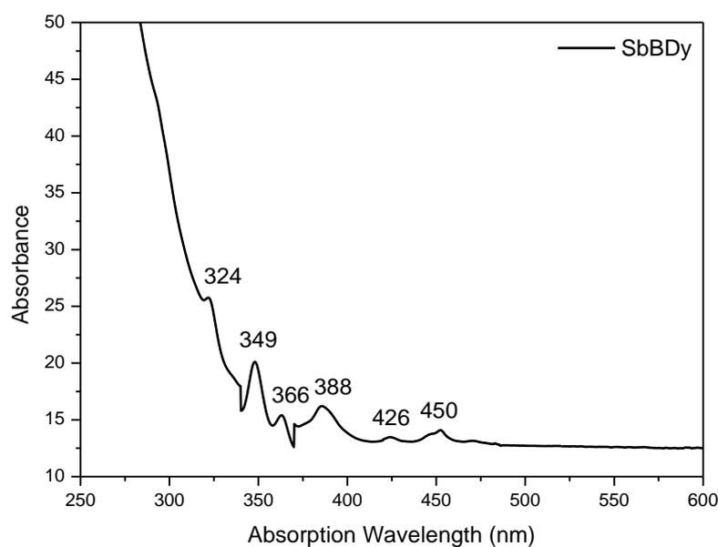
Fig. 1B Optical absorption spectrum of SbBDy0.5 glass
