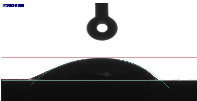
Figure 1d. Mild Steel Immersed In Aqueous Extract of Justicia Adhatoda L Leaves
