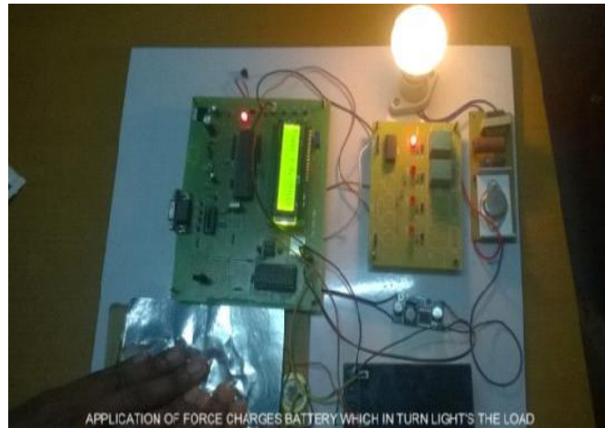
Fig.4. Experimental setup of Foot step power generator system using piezo electric sensors.
