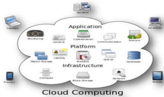
Fig 1.1 Structure of cloud computing
